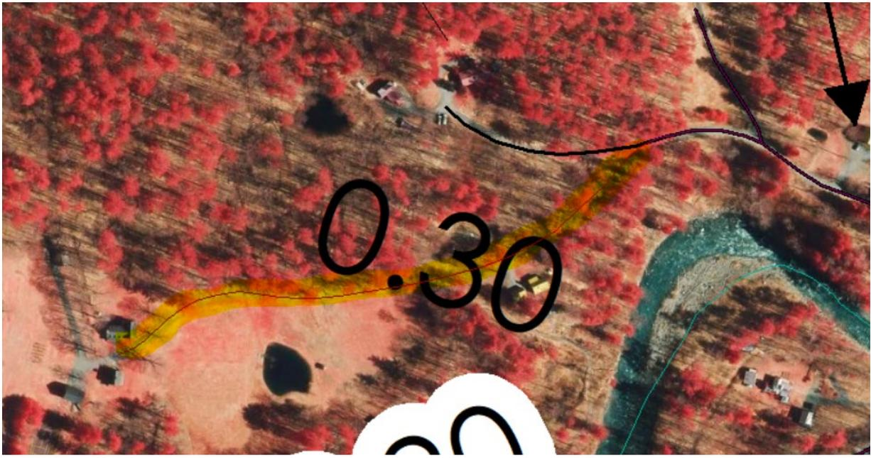
The third road is **LT-11 (Upper Railroad Ln)**. I am rather unsure about the alignment of this road as E911 has it mapped a little differently (pink line) than we do. Looking at the elevation data, it could very well follow either of the yellow highlights below. When looking at this I noticed the intersection of TH-83 and TH-15 should also be updated to show the fork on TH-83 (see 2<sup>nd</sup> image below).
