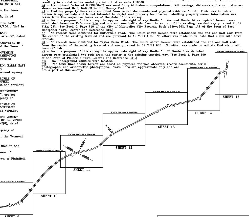
N1 - The Vermont Agency of Transportation authorized the survey of the right of ways, easements, and fee titles associated with Vermont Route 214. This survey was performed in accordance with 19 V.S.A. §33 - Survey of existing highways;
