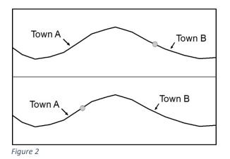
Moving a pseudo node is sometimes required to modify the location where an attribute changes. For example, in Figure 2 a pseudo node needed to be moved to change the location of a town boundary. All of the attributes for the two arcs remain the same; only the location of the pseudo node has changed. This entails splitting and unsplitting the two arcs, and therefore would be coded as 'S' or 'U'.
