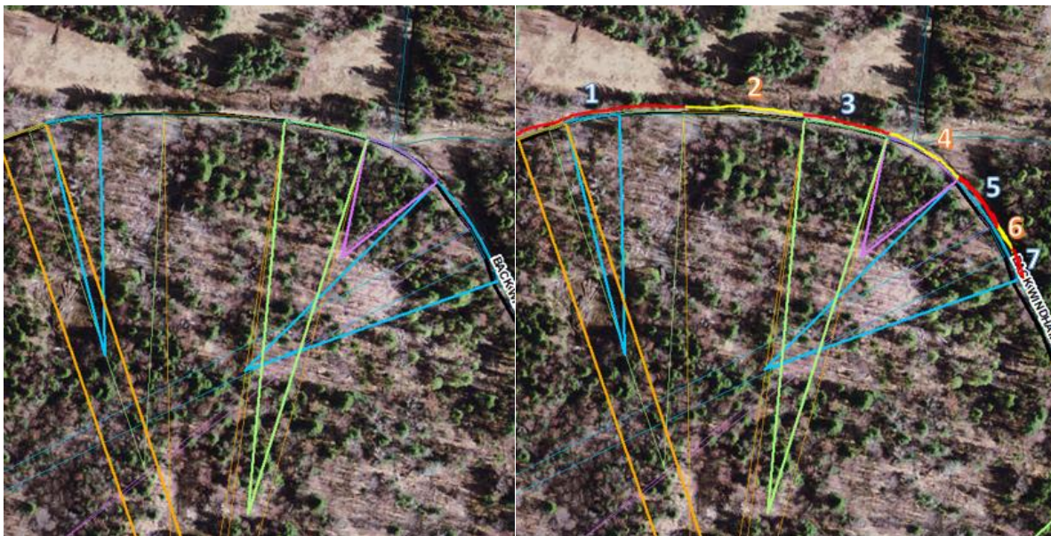
Figure 6 : The eastern portion of Back Windham Road shown in earlier figures, again showing where curve-class has changed after performing quality control edits to the centerline.
