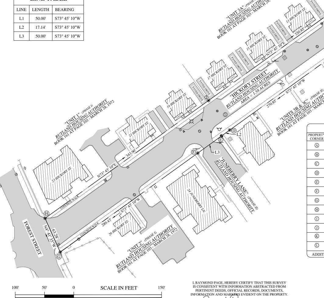
A TOPCON PS 103A TOTAL STATION CLOSED TRAVERSE SURVEY
