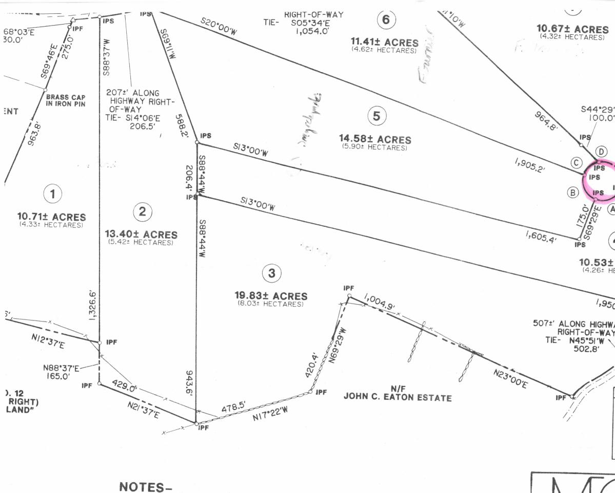
I. THIS SURVEY WAS BY CLOSED AND ADJUSTED THEODOLITE-ELECTRONIC DISTANCE METER TRAVERSE. THE ERROR OF CLOSURE BEFORE ADJUSTING WAS I IN 13.280
